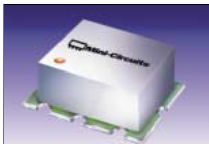
2. The model HJK-21H is a double-balanced FET-based mixer designed for use with RF signals from 1850 to 1910 MHz and LO signals from 2090 to 2150 MHz.
